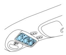
In order for the auxiliary A/C-heater controls to function, the driver's auxiliary A/C-heater control must be set to REAR.
